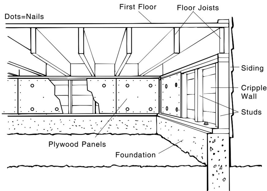
**Figure 3—Plywood strengthens weak cripple walls.** *If your home has a cripple wall between the foundation and the first floor, and the wall is not braced with plywood sheathing, the house may collapse during an earthquake.*
