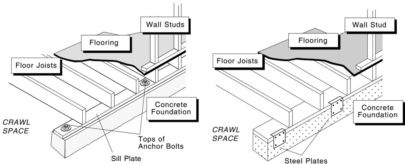
**Figure 2—Anchor bolts or steel plates.** A home's crawl space may be formed by a cripple wall between the foundation and the floor joists (as illustrated in figure 3, page 5) or the floor joists may rest directly on the sill plate. In either case, you should be able to see the heads of anchor bolts or steel plates installed every 4 to 6 feet (not necessarily exactly as shown here). These fixtures fasten the sill plate to the foundation.
