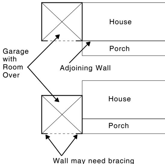
**Figure 5—Additional bracing.** If the wall of the main house is in line with the wall containing the door of a garage with a room over it (top figure), the adjoining wall will help brace the garage. If the “in-line” wall consists only of porch supports (bottom figure), the garage may require additional bracing.
